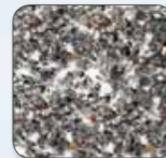
Split and deformed several times. Particle size max. 10 mm<sup>2</sup>
