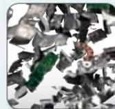
Split and deformed several times. Particle size max. 320 mm<sup>2</sup>
