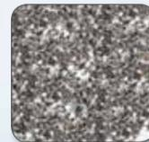
Split and deformed several times. Particle size max. 5 mm<sup>2</sup>
